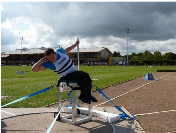
Peter built a wooden prototype seat before finalising the design. It was intended that the basic seat would be adaptable for all athletes, in addition to making seats for specific clients. His final design was based on a rectangular frame of aluminium tube on a square base with the full frame in contact with the ground to minimise sinking into soft ground. A tubular pole for the athlete to hold was attached, its position variable for the different throwing events.
